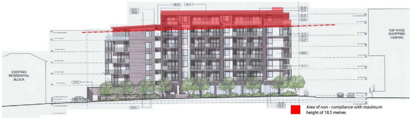
Figure 10 North-west elevation showing non-compliance with maximum 18.5 metre height
